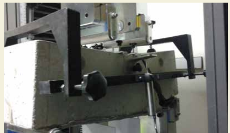
Figure 2: Bending test of CFRP reinforced concrete prism sample
