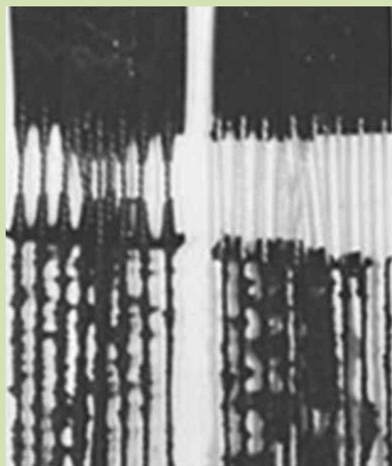
Figure 4: RF-free (left) and RFL treated cords (right) after vulcanisation in rubber compounds
