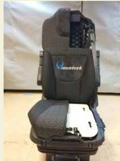
Figure: The prototype of composite seat structure
